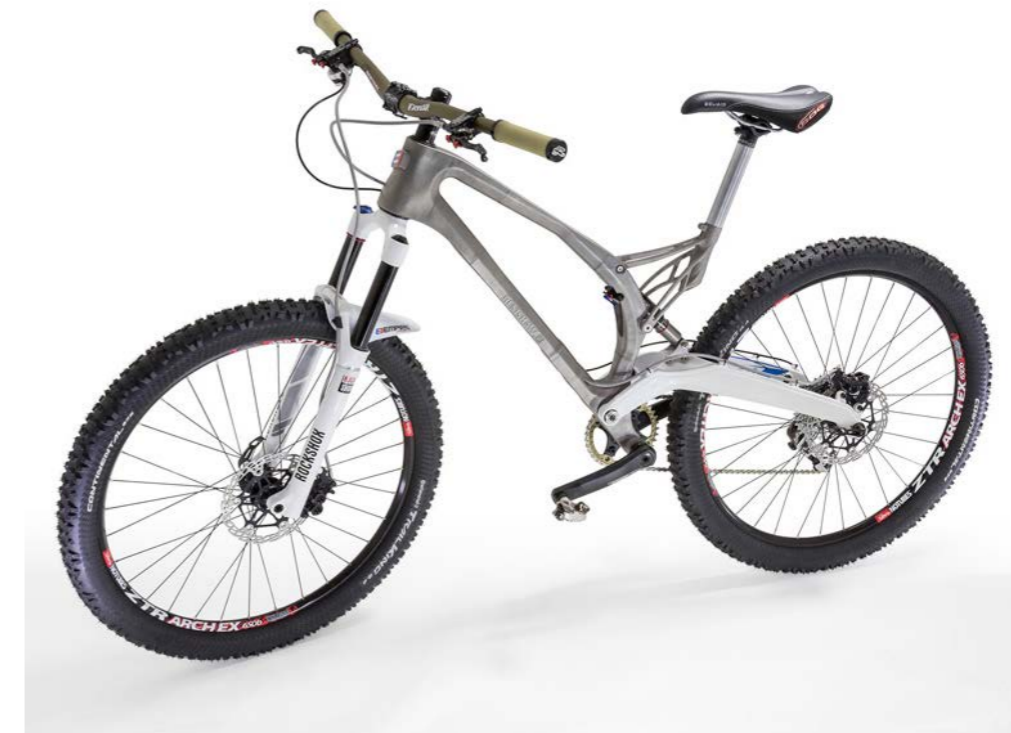
Figure 5.2: Empire's MX6-R, the only 3D printed bicycle in the world with a 33% lighter and six times stronger frame than its aluminium counterpart [42]
